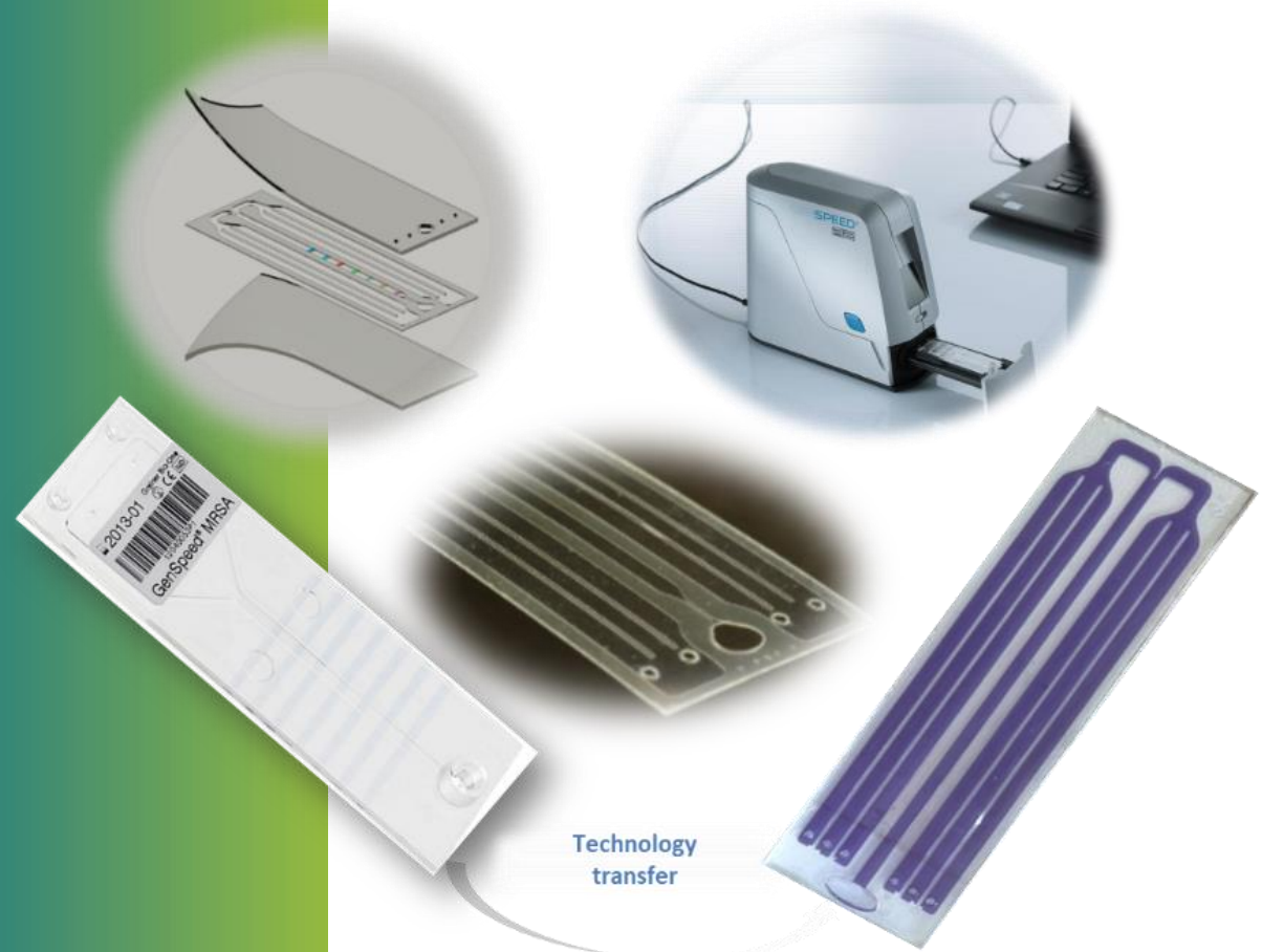
Transfer of fluidic structures from injection molding to R2R-produced \mu F-channels
