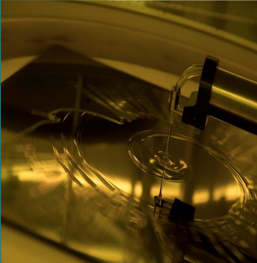
Spincoating of the resin
