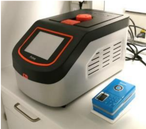
Conventional thermocycler (left) vs pseudo-isothermal PCR cycler (right) (1500bp: 2hours vs. 30min)
