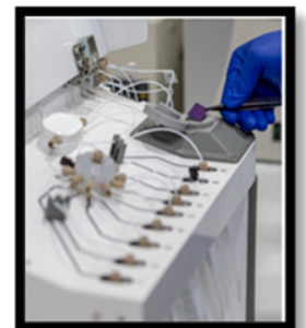
Cellsway chip mounting interface within the benchtop control instrument
